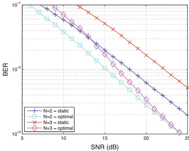
**Fig. 5** Numerical performance in terms of average user BER w.r.t. average SNR for systems with  $N = 2$  and  $N = 3$  users under static and optimal ordering
