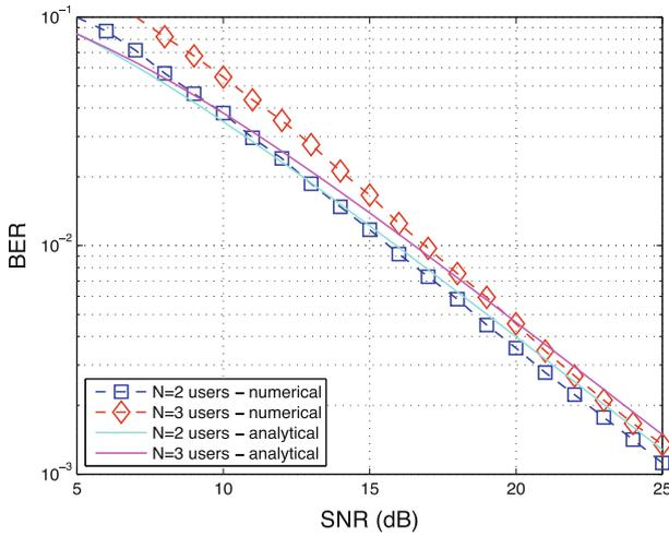
**Fig. 4** Numerical and analytical performance in terms of user BER w.r.t. user SNR for systems with  $N = 2$  and  $N = 3$  users under optimal ordering
