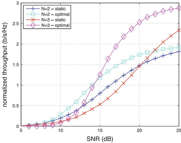
**Fig. 6** Numerical performance in terms of normalized throughput w.r.t. average SNR for systems with  $N = 2$  and  $N = 3$  users under static and optimal ordering
