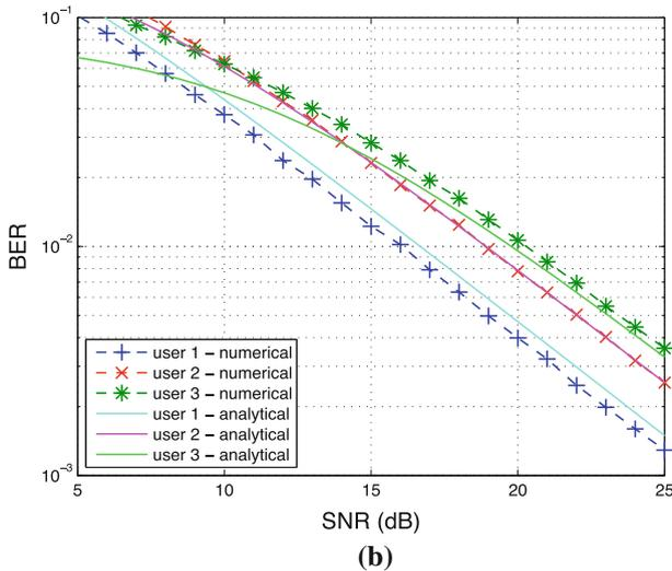
**Fig. 3** Numerical and analytical performance in terms of user BER w.r.t. user SNR under static ordering. **a** System with  $N = 2$  users, **b** system with  $N = 3$  users
